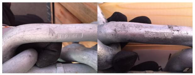
Batch format: V 19 Marked every meter. Letter (V) and number (19) on each chain link. 4 links between letters and numbers.
