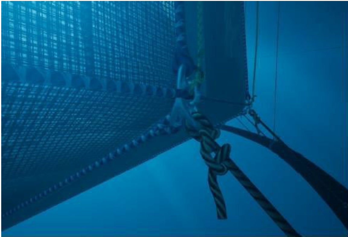
Figure 2: Super Duplex Connection Plate at bottom rope cross-points
