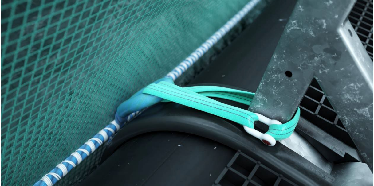
Figure 1: Attachment method with sling and shackle.
