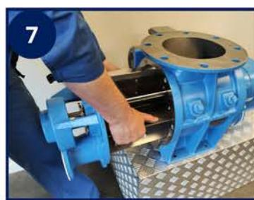
Support the rotor while removing it completely.
