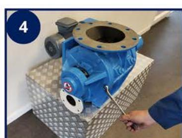
Unscrew and remove the bolts of the end disc at the non-driven side.
