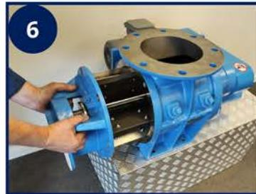
Pull out the rotor half way.
