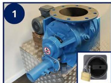
Empty the valve and switch off the power. Lock, tag and try the power switch.
