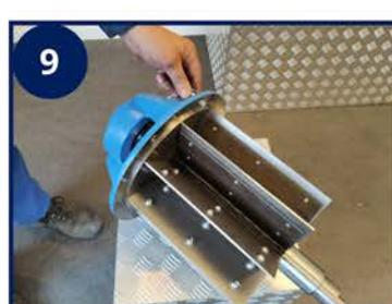
Remove the bolts from the threaded holes.
