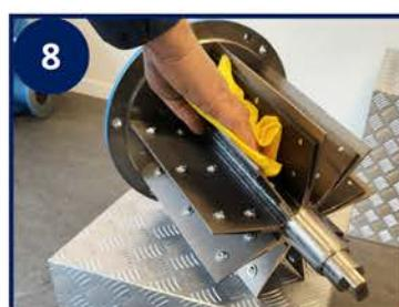
Clean end cover, rotor, shaft and spigot.
