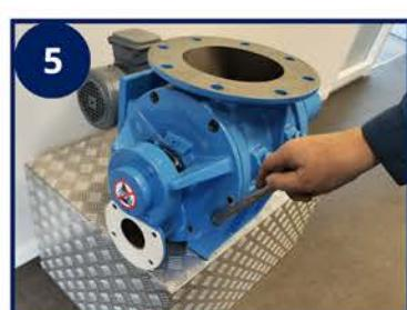
Insert 2 bolts in the threaded holes. Turn evenly to push the end cover from the body.
