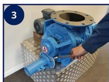
Demount the pipe connection piece at the non-driven side.
