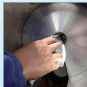
11. Clean seal and shaft area both end covers
