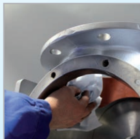
10. Clean valve internally (also inlet)
