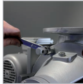
3. Remove bolts non drive side
