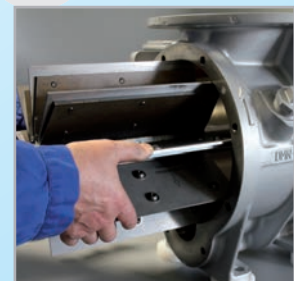
12. Support rotor and replace
