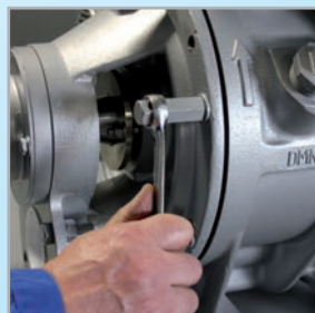
14. Insert and tighten bolts
