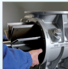
7. Support rotor and remove
