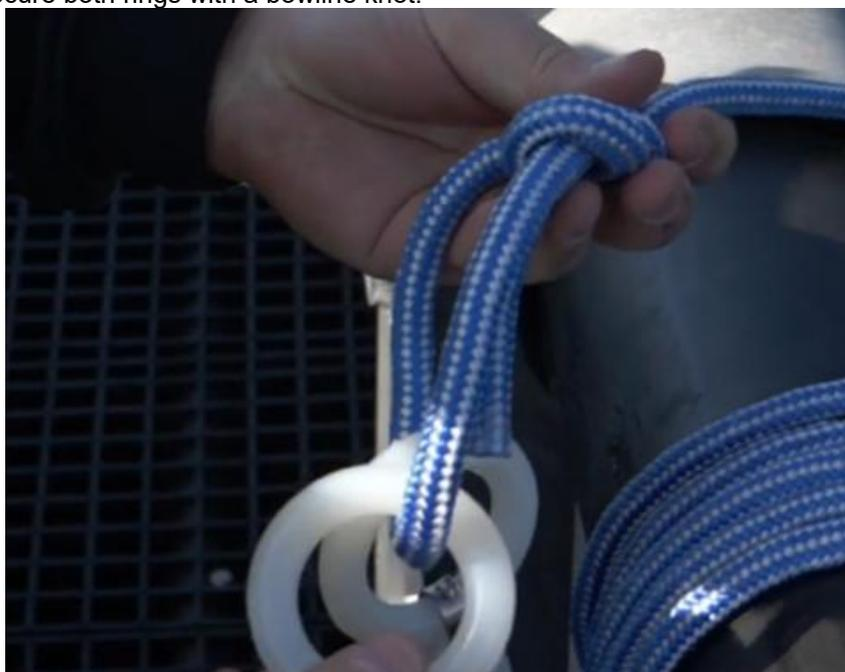
12. Then thread the ring without a pulley over the knot to create a loop that can be threaded onto the winch's wheel.
