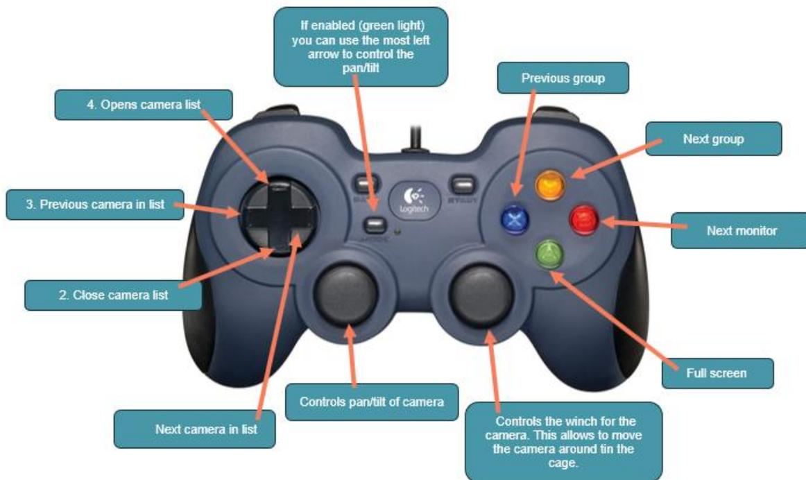
Figure 45 Hand controller top
