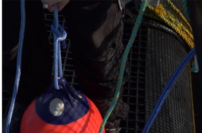
7. If you want to finish the work with the counterweight and make it easier to adjust the length of the winch rope, release the counterweight into the pen. If you want to use an additional means of securing it, you can tie an extra rope to the counterweight and tie it to the support on the ring.
