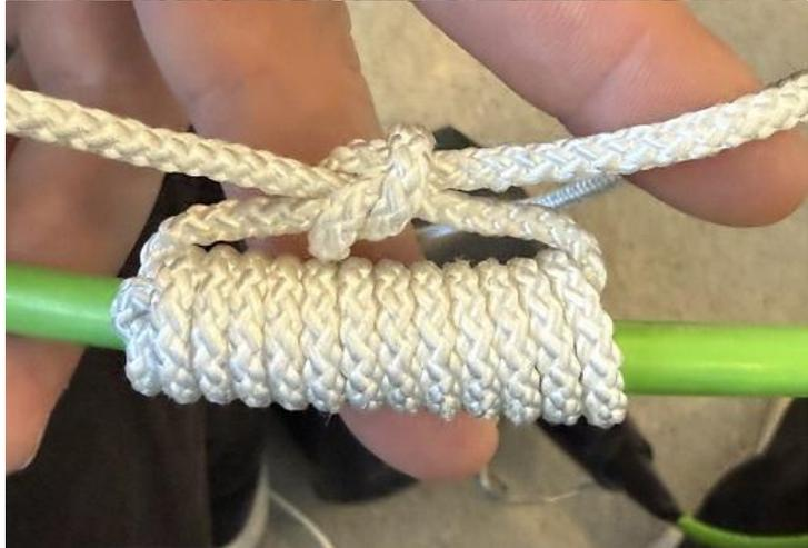
This way, the tension is mainly applied to the bowline knot rather than directly on the cable.
