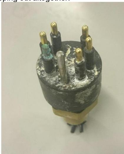
Figure 1 : Underwater plug with corrosion and white coating
