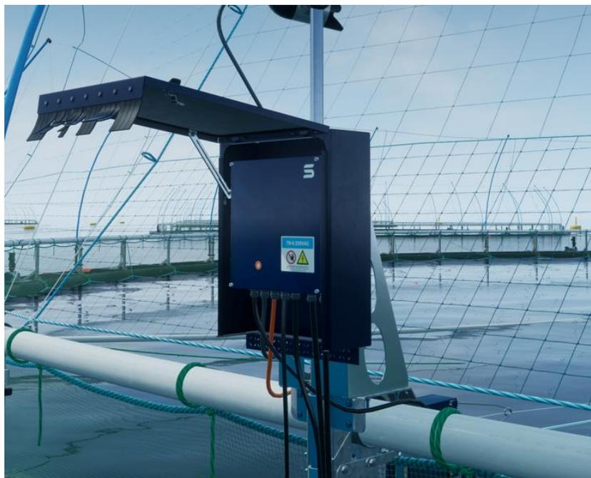
Figure 6 CIU mounted in protective housing
