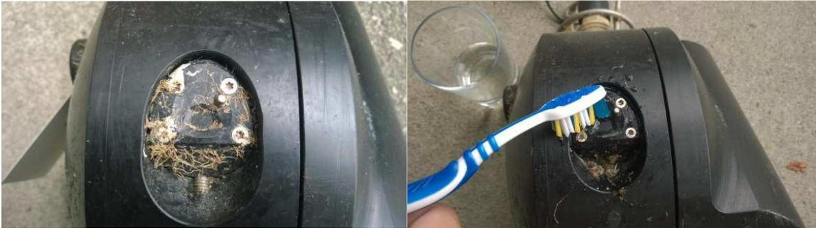
*Figure 51 Cleaning a fouled oxygen sensor on an Orbit-3500 camera*
