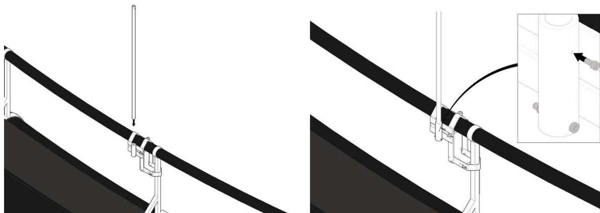
Figure 23 Mount the mast in the mounting bracket and secure it with a set screw.
