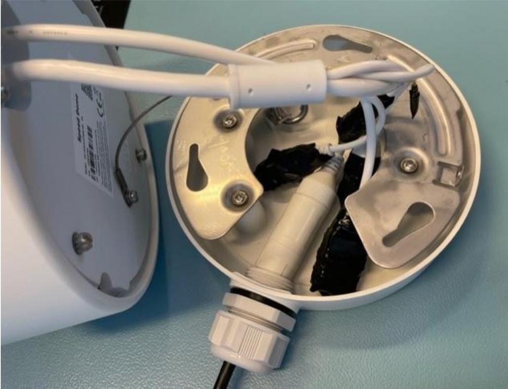
Figure 42 Connector base with all of the cables for the Orbit-360
