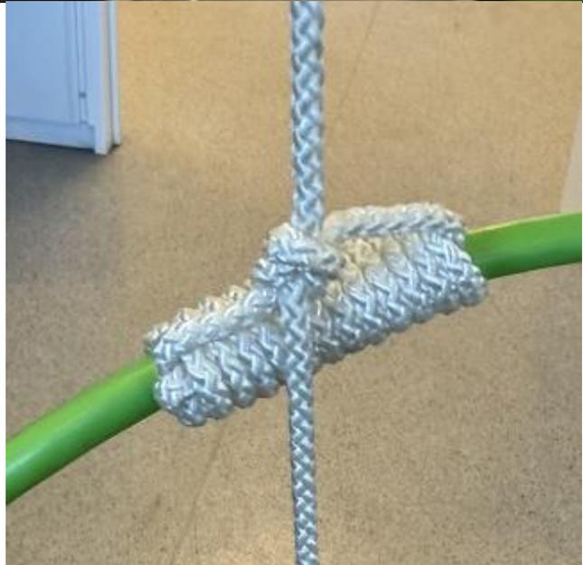
**Step 5:** Secure it to the camera using a bowline knot, with the loop around the camera connector to keep it in place. Make sure the weight is supported by the rope and not the cable.
