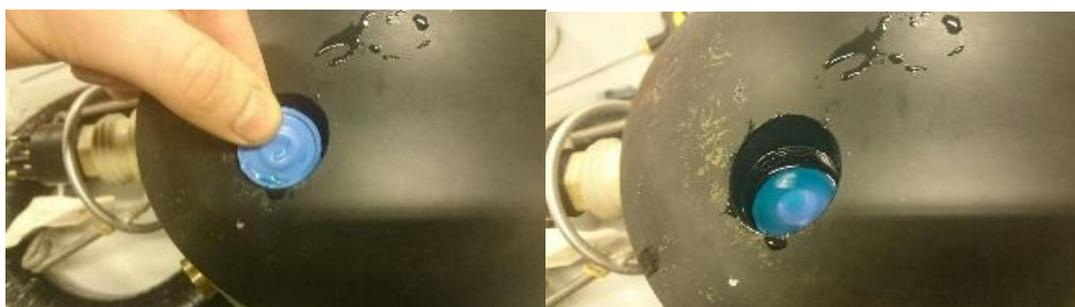
Figure 49 Membrane placement
