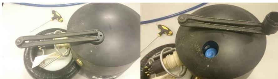
Figure 47 Opening the depth sensor cover
