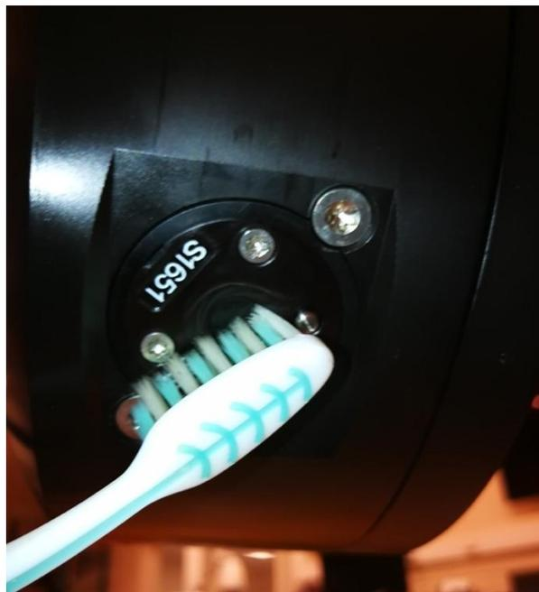
*Figure 52 Cleaning a fouled oxygen sensor on an Orbit-36X0 camera*
