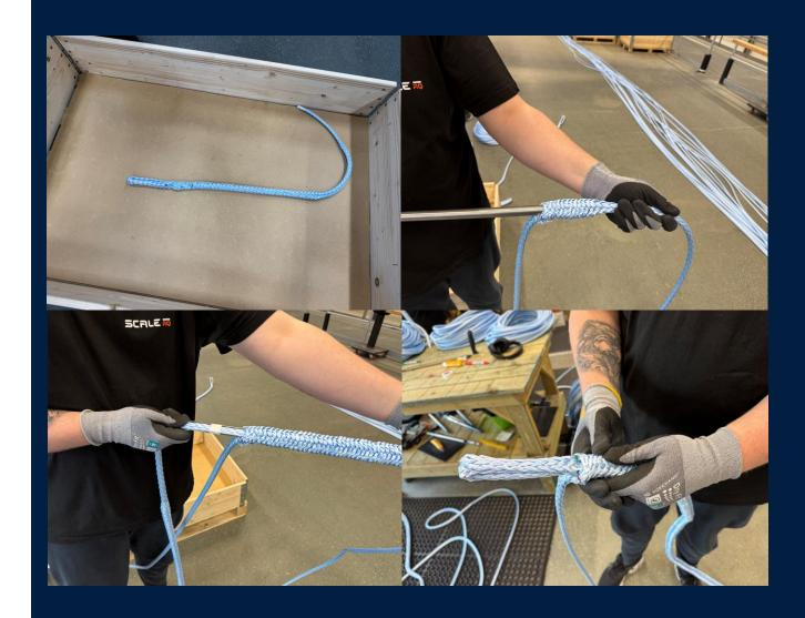
Open the winch rope with a needle and feed the end until the loop stops at the 18 meters mark.
