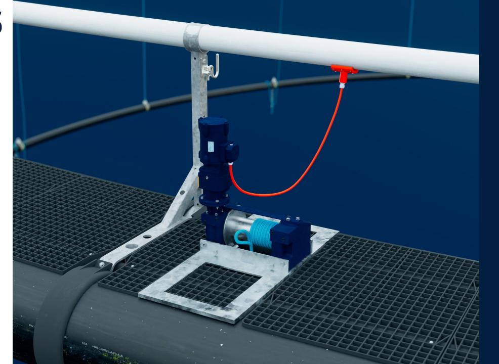
Lower the sinker tube with all winches until the storage loop on the aquaneema rope is accessible for choking. The loop is installed 6 meters from the end of the aquaneema rope.
